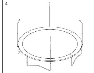
5. Lay out Top G4 Pole (8), joint each section Connector to a straight line as shown.
