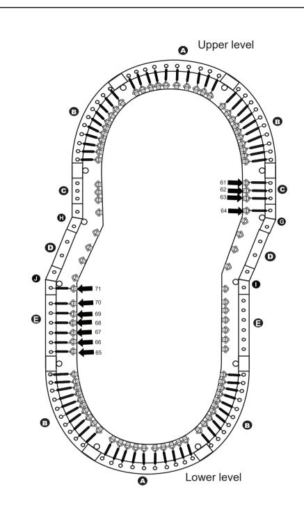
After the springs underneath have been attached, continue attaching the springs (part 26) on remaining top rails.
