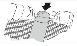
Stand on the trampoline and insert one of the exposed sections of the Black G3 pole into a plastic grip on top of one of the enclosure poles.
