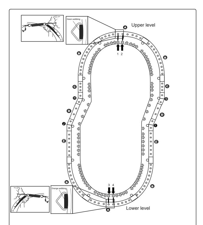
Insert the Closed end of one spring Part 26, onto one of the webbings Green and Orange stitched V-Rings as shown.
