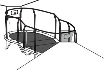
Use 4 pcs Black metal screws to fix the target game through to the enclosure mesh.
