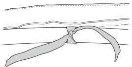
Tie the outer elastic straps on the underside of the frame pad around the top tubes of the frame.
