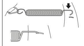
**IMPORTANT:** Springs must be inserted in the correct direction. The closed end will attach to the stitched mat and open end to the frame. Ensure all the springs are fully inserted into the slots on top of the frame.
