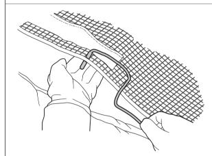
Tie the end of the cord around a V-Ring. Push the end through a hole in the bottom of the netting.
