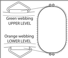
Locate the V-rings with Green webbing for upper level of trampoline.
