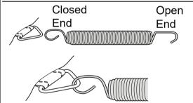
**IMPORTANT:** Identify the closed end of the spring and the open end of the spring for proper assembly.
