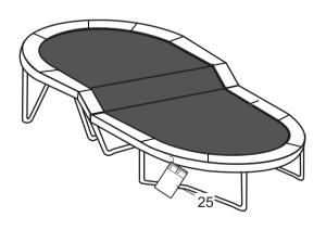
Using the included plastic tie, attach the Safety Placard to the frame near the point where jumpers will climb onto and off the trampoline. The trampoline is now fully assembled. Make sure that all parts are securely attached. Familiarize yourself and all users of the trampoline with the safety precautions, use and instructional materials, and care and maintenance instructions in this manual before using the trampoline.
