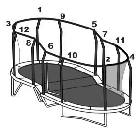
Attach the 11 other exposed sections of the G3 FRP poles to the other enclosure tubes in the order shown in the diagram.
