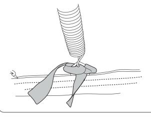
From the underside of the trampoline, tie the remaining elastic straps around the springs or through the V-Rings.
