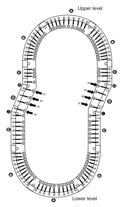
Attach the remaining springs to the top rails according to the number sequence shown in the above images.
