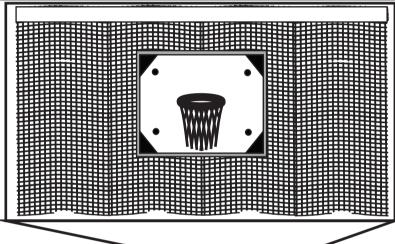
Use 4 pcs Black metal screws to fix the Basketball mesh through to the enclosure mesh.
