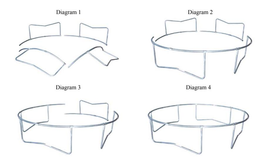
Diagram 1: Now take two sections of completed legs and flip them over and rotate them 180°. Diagram 2: Next, connect these two sets of legs together at the T-connector of one and the open tube of the other. Diagram 3: Now, flip over, rotate, and connect the next leg set to the complete previous sets. Diagram 4: Finally, flip over, rotate, and connect the final leg set to complete the ring of the trampoline frame.
