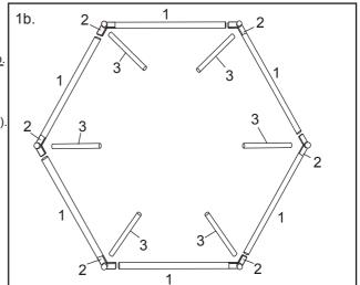
1b. You have now assembled one leg sections. Repeat the step to assembled remaining sections.
