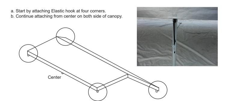
IMPORTANT! Once the legs and cover are assembled, your canopy will be proned to wind damage. It is imperative that the canopy anchors be installed NOW!
