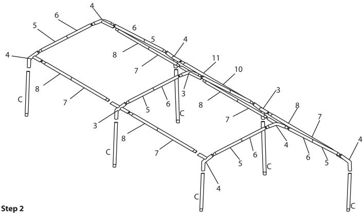
Start with the center and complete the center frame first. Then assemble each side.
