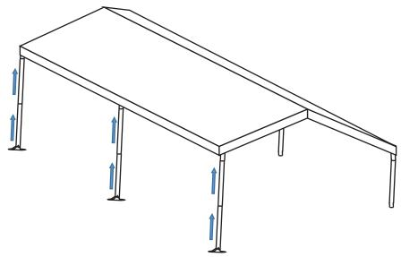
**Step B:** Connect the hook down to the Top leg frame(C) of each leg.
